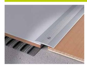
STRIPTEC ST profiles are designed to join adjoining floors of equal or different type and thickness. The rounded shape of this profile covers edge imperfections and allows a slight rotation, compensating for elevation differences of up to 3/16" (5mm). It can also be used as a termination profile, given a floor thickness of up to 3/16" (5mm). Available in two versions: selfadhesive and screw-on.
